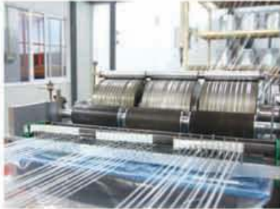
Pressure tanks are made of high performance Composite material with Fiber glass filament winding
